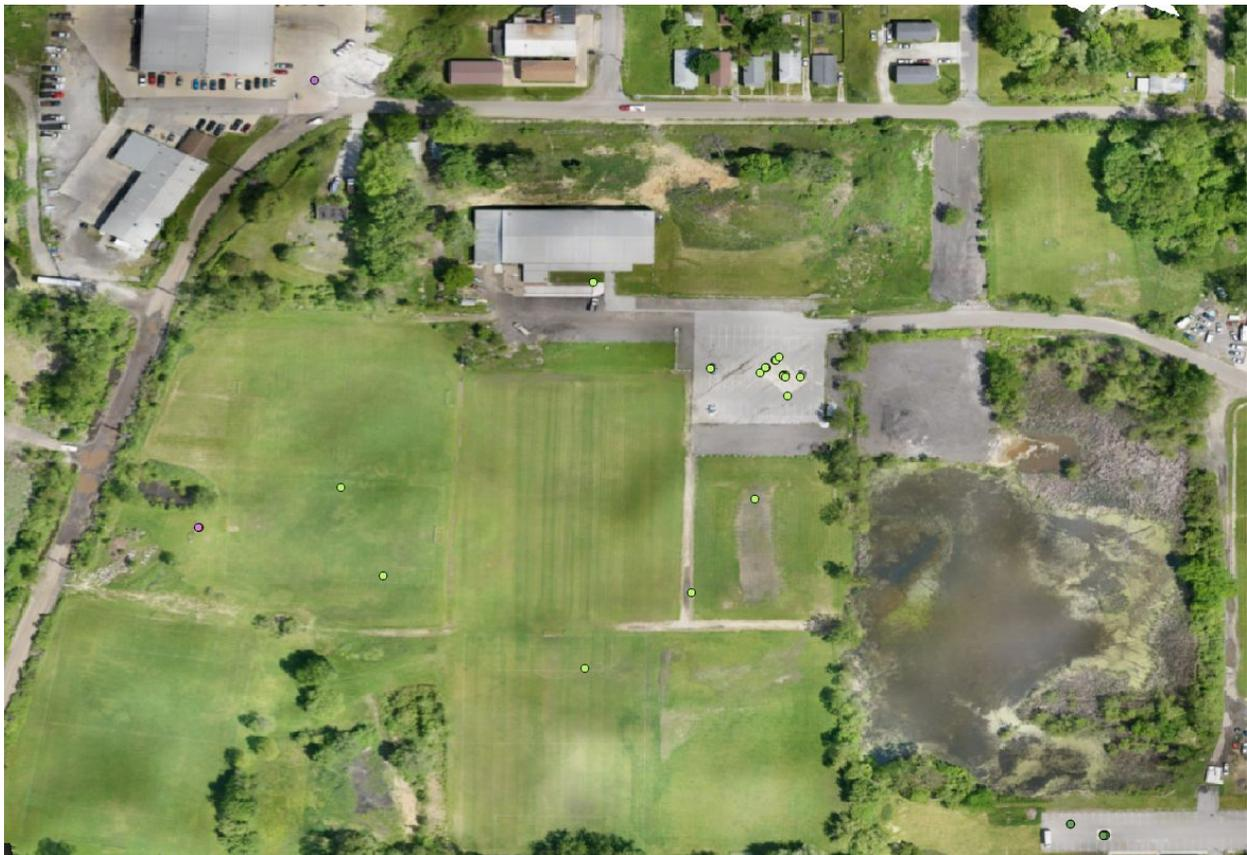
Agisoft Photoscan Professional version 1.4.2 was used to post-process the imagery and create an orthomosaic and digital elevation model (DEM). Settings used to post-process the imagery are recorded below in Table 4.
